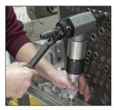
Standard locking system with handle feed makes quick work of trimming back tubes.
