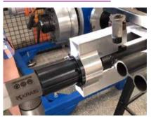
PanelDrill during 2" carbon steel membrane removal.
