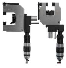
PanellMill-PF is available in two versions: right angle and in-line. You can choose the version, which suits better for your needs. Both models have exactly the same parameters.
