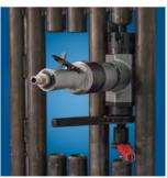
PrepMill with its 66 mm (2-5/8) width body perfectly fit into limited access areas such as Water wall panels. Easy to clamp and feed with our heavy duty ratchet or star wheel feed.
