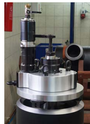
Machining pipe 18" schedule 160
