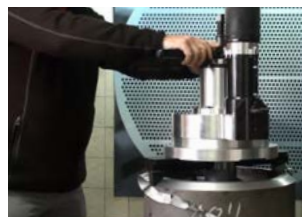
ID Clamping End Prep Tool 4" I.D. to 19" O.D. 101,4 mm I.D. to 500,0 mm O.D.
