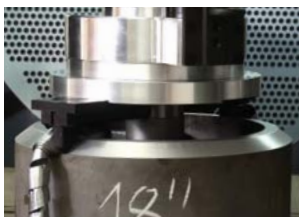
ID Clamping End Prep Tool 4" I.D. to 19" O.D. 101,4 mm I.D. to 500,0 mm O.D.
