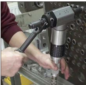
Standard locking system with handle feed makes quick work of trimming back tubes.
