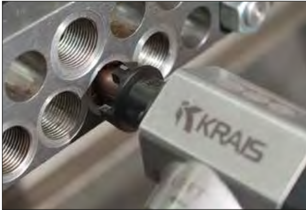
☞ Safely re-machine gasket surfaces in seconds.
