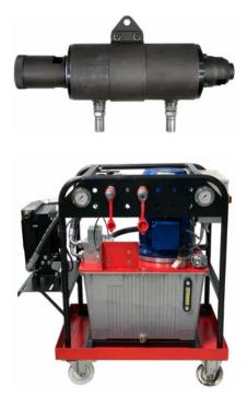
The KRAIS ACTP is an automatic and very fast pump and pulling gun set, is designed for continuous, and stub removal of tubes from boilers, condenser and heat exchangers.
