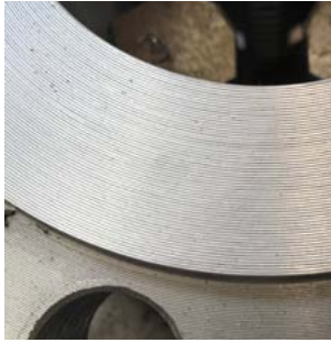
Single line gramophone groove (50 grooves per 1 inch)
