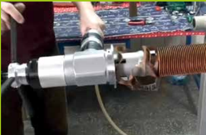
Removes 4.0" (101 mm) depth of fin from the tube OD in less than 2 minutes
