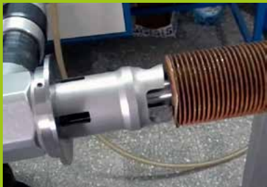
Removes 4.0" (101 mm) depth of fin from the tube OD in less than 2 minutes
