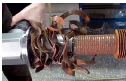
Removes 4.0" (101 mm) depth of fin from the tube OD in less than 2 minutes
