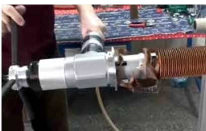
Removes 4.0" (101 mm) depth of fin from the tube OD in less than 2 minutes
