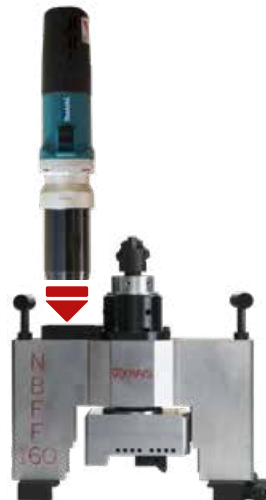
Example of really tight flange – NBFF is the only tool suitable here.
