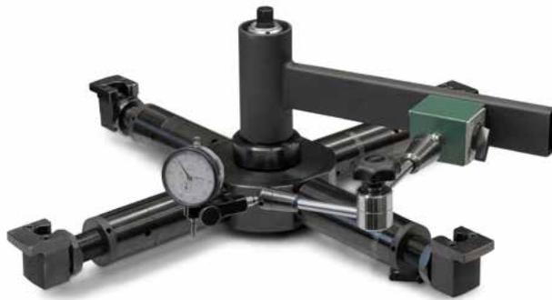
Fast mounted arm with spindle for the very convenient measure of levelling and cantering
