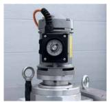
As an alternative, we offer an electric drive for IMFM40&60. The motor provides similar parameters to the pneumatic one.
