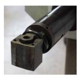
Both machines are equipped with special jaw set for easy, quick levelling and centering. A special mechanism allows convenient adjustment of the mounting plane relative to the pipe. Built-in self-centering locking system significantly facilitates the coarse setting of the machine.
