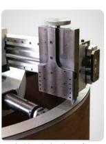
Standard configuration of IMFM is equpped with swivel tool post for grooves, RTJ flanges and bevels
