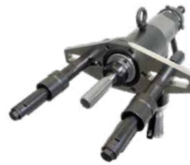
REAMMING Safely ream tube sheets.
