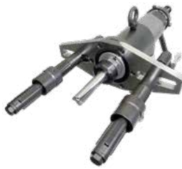
WALL REDUCING Tube wall reducing head with carbide inserts.
