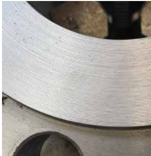
Single line gramophone groove (50 grooves per 1 inch)
