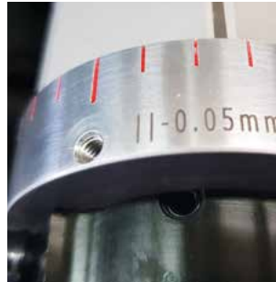
Graduation of the tool setting to the desired depth of cut.
