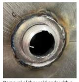
Removal of the weld ends with a visible groove between the tube and the tube sheet.
