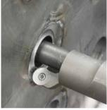
The bit edge covers the entire weld to be removed
