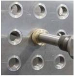
The machine is designed for work on gas coolers: an elongated special head and a nut fixing the tool in the socket.
