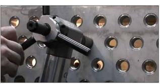
Trimming tubes safely and efficiently. Machine locks securely both to the tube and the plug thread of the water box.
