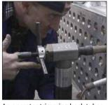
An operator trimming back tubes prior to seal welding.
