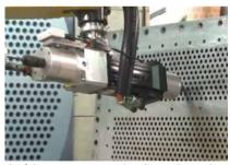
Simultaneous machining of two (!) tube sheets. Both of them were prepared earlier and now they need tube facing and expanding. After on hour setup, all work is done totally automatically.
