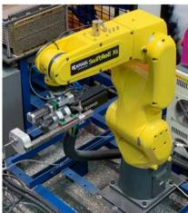
SwiftRoll XS the smallest version of the SwiftRoll. Designed for small cooler manufacturers. With this version, the tube facing is not available. Available motors up to 6000 rpm.
